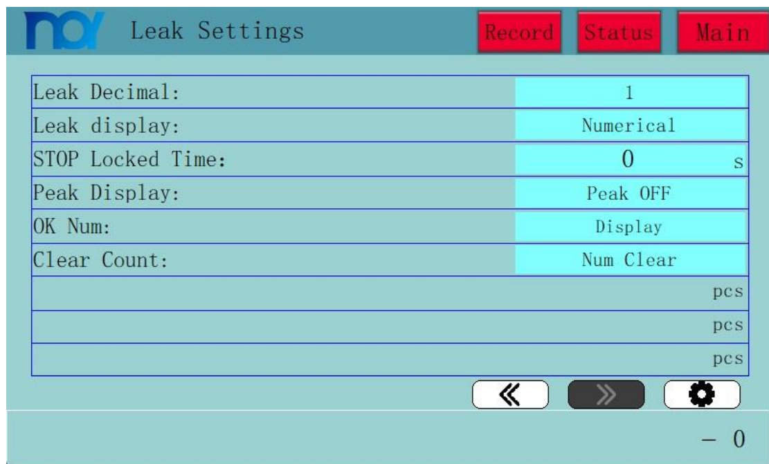
Figure 17 Leak detection setting interface 4
